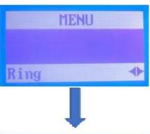
Using the Scroll Left-Right will choose the alert call chime (Melody) and the scroll up-down will adjust the volume of the corresponding alert call chime.
