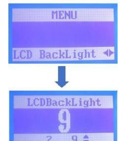
Using the scroll up-down (13) or pressing number 2 to 9 will choose one of the 8 preset backlight intensity levels.
